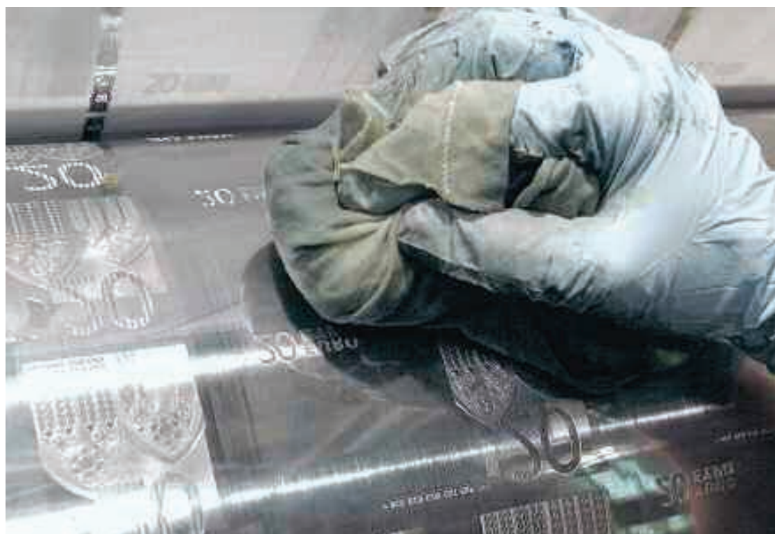
One of many steps in printing a banknote: the intaglio printing plate mounted on a printing roll is being cleaned.
